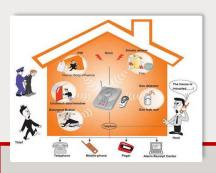
• Intruder/burglar alarm system is a set of interconnected devices that is aimed to protect an object, usually a facility, against intruders and to notify the owner or/and the monitoring station/center of any violation of the protected zones.
